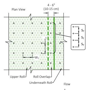
• Twist Pin, HS/HC/HR-8/12, as appropriate for field conditions
