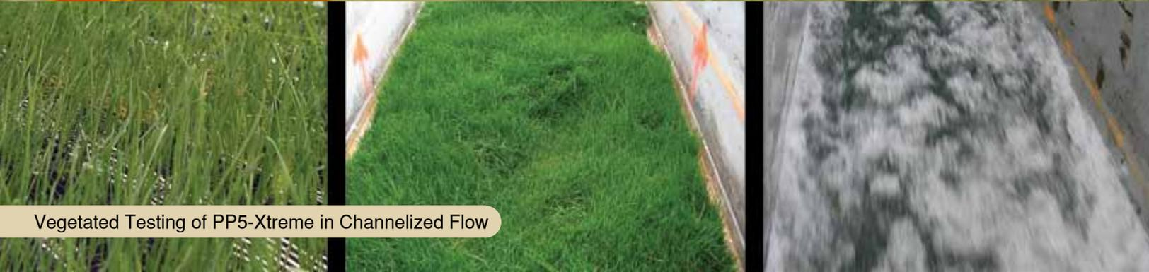
Vegetated Testing of PP5-Xtreme in Channelized Flow
